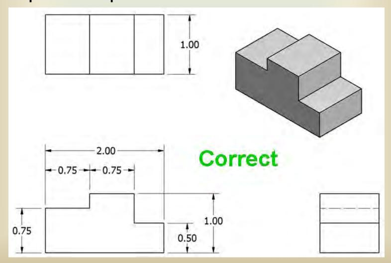
Dimensions should be attached to the view that best shows the *contour* of the feature to be dimensioned.
