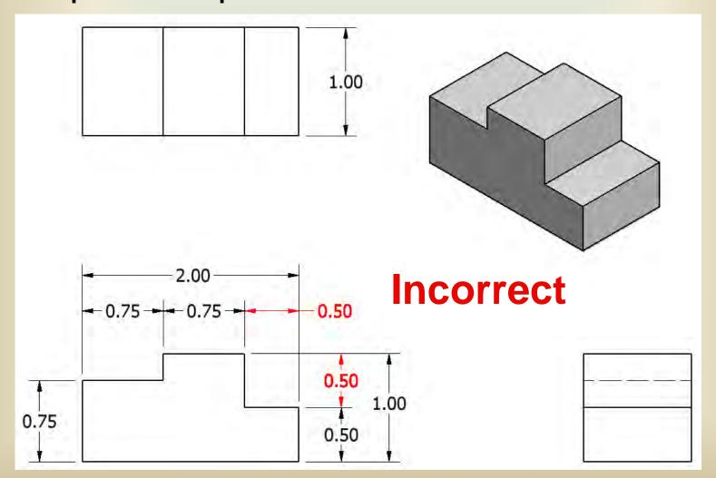
No unnecessary dimensions should be used – only those needed to produce or inspect the part.
