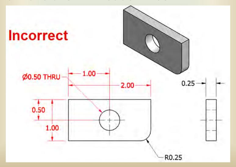
13. Do not cross a dimension line with an extension line, and avoid crossing dimensions with leader lines.
