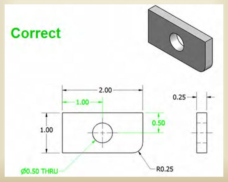
13. Do not cross a dimension line with an extension line, and avoid crossing dimensions with leader lines.
