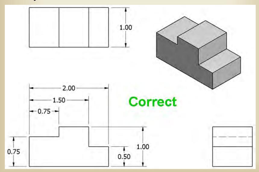
6. A dimension should be attached to only one view; for example, extension lines should not connect two views.
