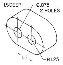
2. Sketch the following object in Inventor. Then create a drawing with the views necessary to describe the object. Dimensions are in inches.
