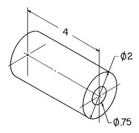
2. Sketch the following object in Inventor. Then create a drawing with the views necessary to describe the object. Dimensions are in inches.
